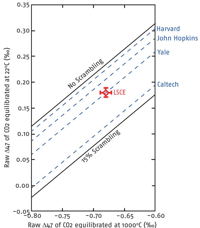
Fig. 1: Comparison between IsoPrime measurements and inter laboratory data from Dennis et al.2011
